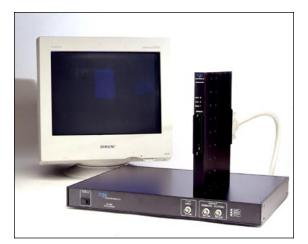
Model PC-1800 multi-channel SQUID electronics (monitor not included)
