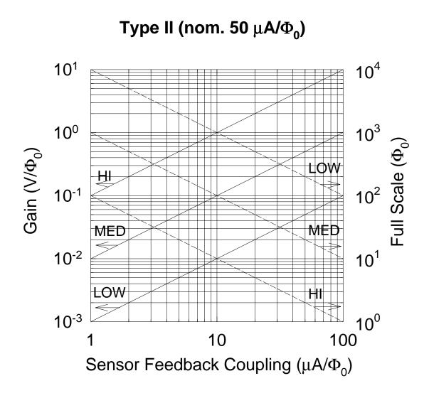
Figure 5-4. Feedback loop gain and full scale range as a function of sensor feedback coupling with the PFL-100 programmed for Type II SQUIDs which have a nominal 50  $\mu$ A/ $\Phi_0$  coupling. In this case, the feedback resistors for the sensitivity ranges 'High', 'Medium' and 'Low' are equal to 100 k $\Omega$ , 10 k $\Omega$  and 1 k $\Omega$ , respectively.
