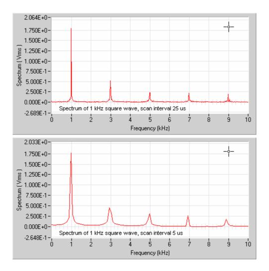
Figure 4-11. Dependence of the computed spectrum on the scan interval. The interval is 25  $\mu$ s for the upper graph, and 5  $\mu$ s for the lower graph. The number of data points is 2048 in both cases.
