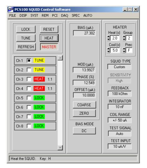
Figure 4-3. Appearance of the main panel of the SQUID Control Module during a heat cycle. Only the heater controls and the State indicators can be operated while heating or cooling is in progress. The Count indicators show the amount of time left for heating (1.5 sec). Here the system is in the Master mode (see Section 4.2.8), and channels are heated in groups of two.
