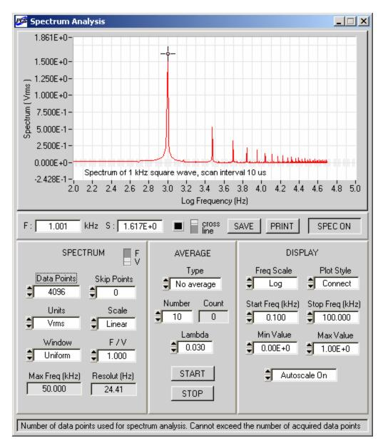
Figure 4-10. Typical appearance of the Spectrum Analysis panel. The "Max Freq" indicator displays the maximum frequency which may be probed for the selected scan interval. The "Resolut" indicator shows the corresponding frequency resolution.
