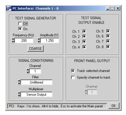
Figure 4-4. The PCI panel for channels 1 to 8.
