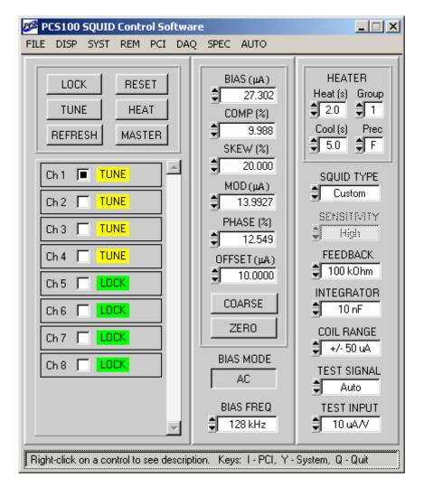
Figure 4-2. Appearance of the main panel of the SQUID Control Module if the selected channel is operated in the AC bias mode. The COMP, SKEW, and BIAS FREQ controls are now visible and functional.
