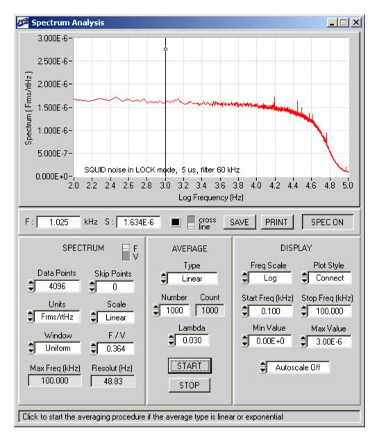
Figure 4-13. Spectral density of a SQUID operated in the LOCK mode. The engineering unit F is the flux quantum, and the ratio 0.364  $\Phi_0/V$  is the calibration factor. The displayed curve corresponds to the linear (RMS) average of 1000 individual spectra.
