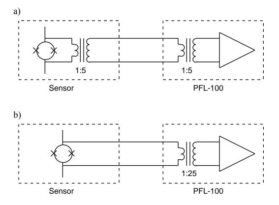
Figure 5-1. Transformer coupling options for the PFL-100. a) Dual transformer coupling. b) Single transformer coupling. Note: In the single-transformer configuration, a blocking capacitor (not shown in the figure above) is used to prevent the shunting of the SQUID bias current by the warm transformer primary.
