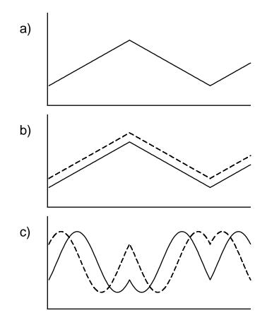
Figure 3-1. Effect of the OFFSET adjustment on the SQUID output in the TUNE mode. a) Test signal vs time. b) Flux applied to sensor vs time: the solid line corresponds to OFFSET = 0, the dashed line corresponds to OFFSET > 0. c) SQUID output vs time for this applied flux: the solid line is for OFFSET = 0, the dashed line is for OFFSET > 0. In these figures, the test signal peak-to-peak magnitude corresponds to  $1 \Phi_0$ .
