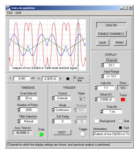
Figure 4-7. Data acquisition from three channels using a PCI-6034E board. The input range and certain display settings are exhibited for the selected DAQ channel by the "Channel" control.
