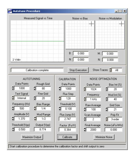
Figure 4-17. Appearance of the Autotune Procedure panel at the end of the calibration. The "Factor" indicator displays the calibration factor determined as a result of this procedure.
