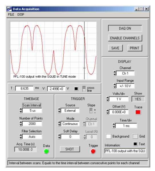
Figure 4-6. Appearance of the Data Acquisition panel using a PCI-6034E board. Only one channel is enabled. The minimum scan interval of 5  $\mu$ s corresponds to 200 kS/s sampling rate.
