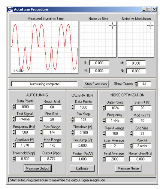
Figure 4-16. Appearance of the Autotune Procedure panel when autotuning is completed. The "Output" indicator displays the final magnitude of the PFL output voltage. Here, the bias search interval is from 0 to 1/4 of the maximum bias value, and the modulation search interval is from 0 to 1/2 of the maximum modulation.
