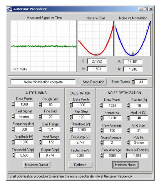
Figure 4-18. Appearance of the Autotune Procedure panel when the noise optimization is completed. The "Noise" indicator displays the noise spectral density at the optimum working point at 1 kHz.
