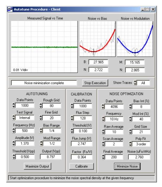
Figure 4-21. Results of the autotuning, calibration, and noise optimization procedures for the same LTS SQUID as in Figure 4-18, but with noise optimization at 10 Hz frequency.
