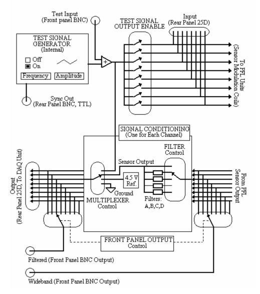
Figure 4-5. Block diagram of the PCI-1000 Interface, showing basic signal routes and their relationship to the PCI panel features. Note that this is a relational diagram only. Some features such as buffers, etc., have been omitted for clarity, and wired connections cannot always be interpreted literally.
