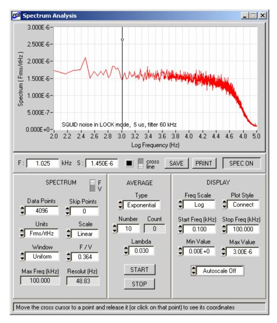
Figure 4-14. The same spectrum as in Figure 4-13, but averaged continuously using the exponential average with  $\lambda$ =0.03. The "S" indicator shows the current value of the exponential average at the spectrum point closest to the vertical line cursor.
