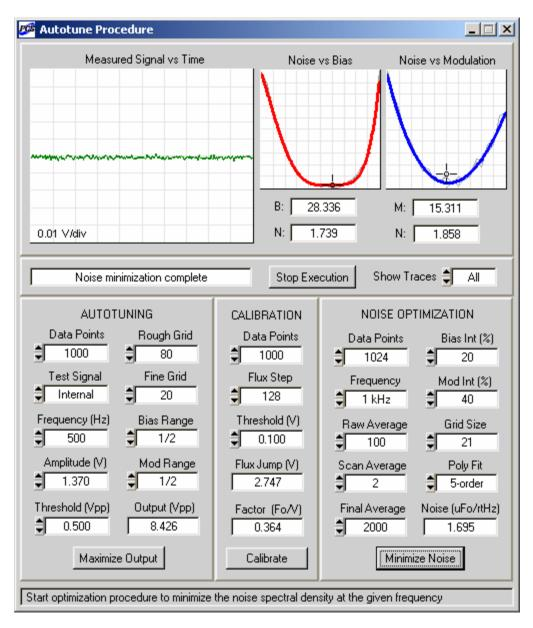
Figure 4-19. Results of the autotuning, calibration, and noise optimization procedures for the same LTS SQUID as in Figure 4-18, but in the AC bias mode with 64 kHz bias frequency.
