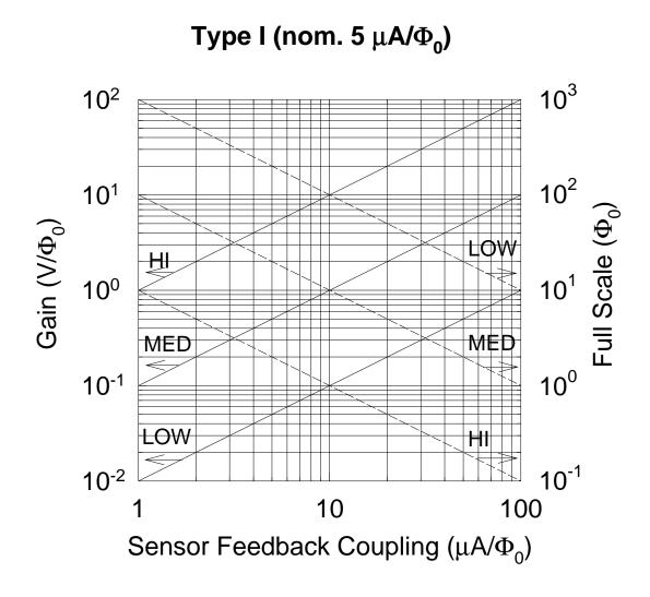
Figure 5-3. Feedback loop gain and full scale range as a function of sensor feedback coupling with the PFL-100 programmed for Type I SQUIDs which have a nominal 5  $\mu$ A/ $\Phi_0$  coupling. In this case, the feedback resistors for the sensitivity ranges 'High', 'Medium' and 'Low' are equal to 1 M $\Omega$ , 100 k $\Omega$  and 10 k $\Omega$ , respectively.
