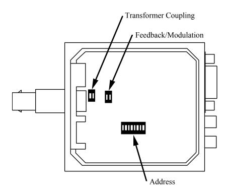
Figure 5-2. Locations of the transformer configuration switch, feedback/modulation connection switch, and the address switch within the PFL-100. Note that in the case of the address switch only, the ON setting actually corresponds to a binary 0 (see text in Section 5.12).
