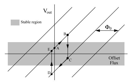
Figure 3-2. PFL-100 output voltage  $V_{out}$  in LOCK mode as a function of the applied offset flux. The output voltage is a multi-valued function shown by the family of diagonal lines. The slope of these lines is the SQUID calibration factor in units of  $V/\Phi_0$ .
