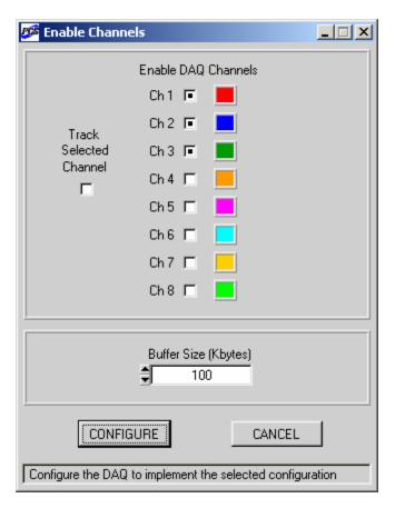
Figure 4-8. The Enable Channels panel of the Data Acquisition Module. Channels 1, 2, and 3 are enabled here. The default buffer size for acquired data is 100 Kbytes.
