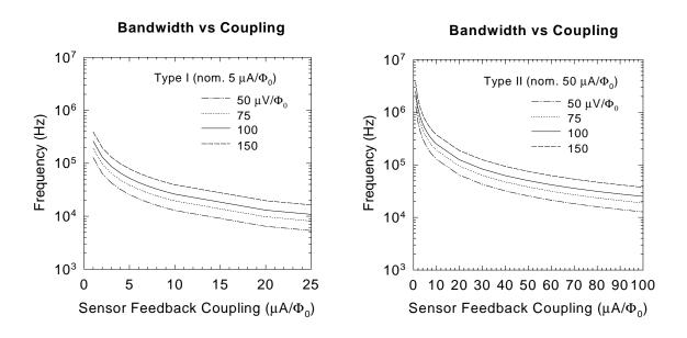
Figure 5-5. The -3dB cut-off frequency as a function of sensor feedback coupling for SQUID Types I and II and several values of the transfer function  $\partial V/\partial \Phi$ .
