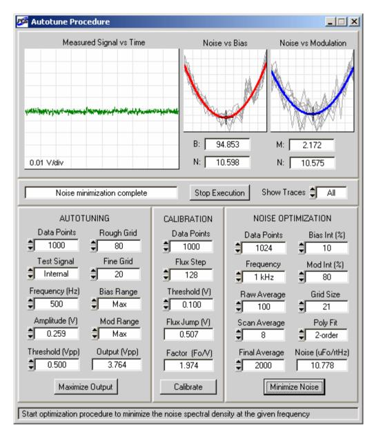
Figure 4-20. Results of the autotuning, calibration, and noise optimization for an HTS SQUID sensor in the AC bias mode with 128 kHz bias reversal frequency.
