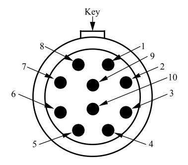
Figure 5-6. The pin numbering scheme for the sensor input connector (LEMO plug style) on the PFL-100, as seen when looking into the connector on the PFL-100.
