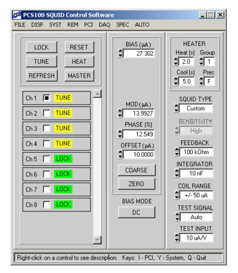
Figure 4-1. The main panel of the SQUID Control Module, configured for 8-channel operation. Channel 1 is the selected channel. It is operated here in the DC bias mode. All control settings on the middle and right sub-panels correspond to this channel. SQUID channels 1 - 4 are in the TUNE mode, while channels 5 - 8 are in the LOCK mode.
