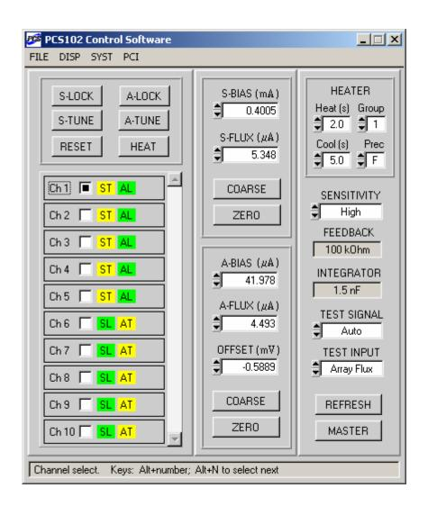
Figure 4-1 The Main panel for 10-channel operation. Channel 1 is the selected channel. All settings displayed on the right correspond to this channel. The first five channels have the input SQUIDs in the TUNE mode ("ST"), and the output arrays in the LOCK mode ("AL"). For the next five channels, the SQUIDs are locked ("SL"), with the arrays in the TUNE mode ("AT").
