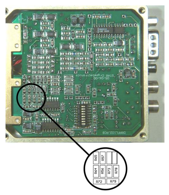
Figure 5-8 Locations of the resistors to set the maximum SQUID and array bias current ranges.
