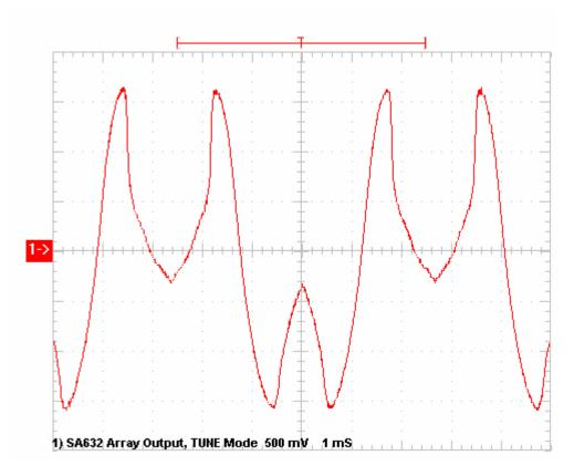
Figure 3-2 Time trace of the PFL-102 output with the array in TUNE mode. A test signal with peak-to-peak magnitude corresponding to 1  $\Phi_0$  is used to modulate the array.
