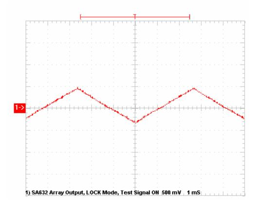
Figure 3-3 Output of the PFL-102 in LOCK mode. The output voltage tracks the applied test signal, which is used to modulate the array.
