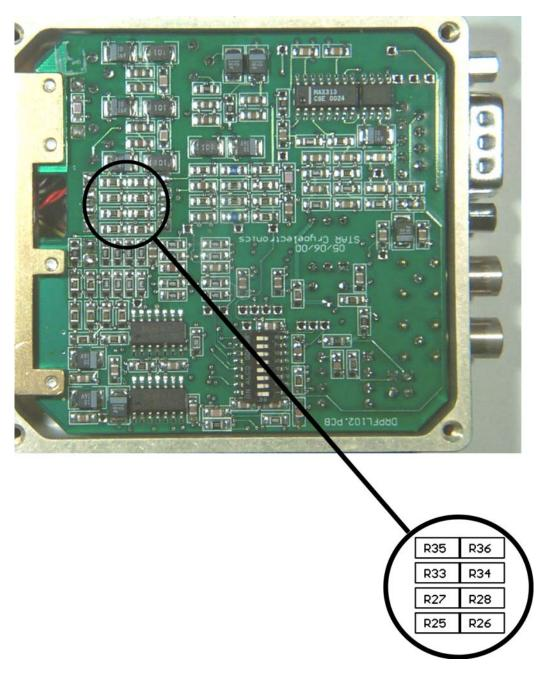
Figure 5-10 Locations of the resistors to set the maximum SQUID and array flux bias current ranges.
