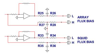
Figure 5-9 Flux bias circuit schematic for the input SQUID and output array. The default values are as follows: R25 and R27 are 40.2 k $\Omega$ , R33 and R35 are 90.0 k $\Omega$ , and R26, R28, R34, and R36 are 10.0 k $\Omega$ .
