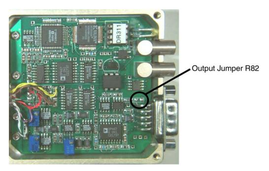
Figure 5-2 Location of the jumper pads to reconfigure the PFL-102 to enable front panel output at the PCI-100 or PCI-1000 interfaces.
