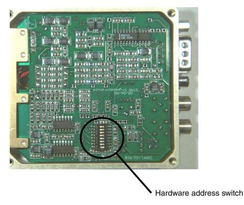
Figure 5-1 Location of the 8-pole DIP switch used to configure the PFL-102 hardware address.
