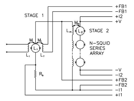
Figure 3-1 Schematic diagram of a typical two-stage SQUID amplifier.
