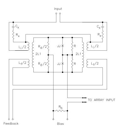
Figure 3-6 Schematic diagram of the input SQUID stage of STAR Cryoelectronics' SA1*xx*/SA6*xx* series SQUID amplifiers.
