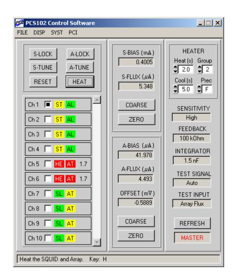
Figure 4-2 Appearance of the Main panel during a heat cycle. Only the heater controls and the State indicators can be operated while heating or cooling is in progress. Here the system is in the Master mode (see Section 4.2.8), and the channels are heated in groups of two.
