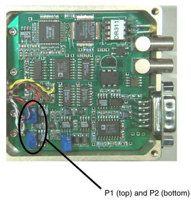
Figure 5-4 Location of the trim pots P1 and P2 used to adjust the input preamplifier balance.
