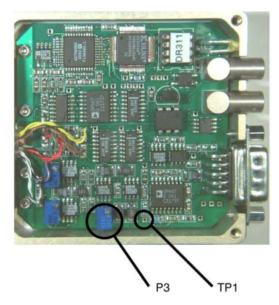
Figure 5-5 Location of the trim pot P3 used to adjust the common mode rejection and test point TP1.
