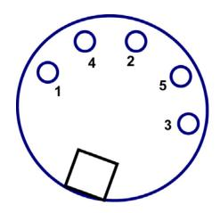
Figure 6-1 Pin assignments for the DIN 5-pin power connector on the rear panel of the PCI-100.
