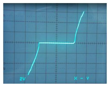
Figure 3-5 Voltage-Current characteristic of the output array of a SA632 amplifier. The output voltage of the PFL-102 is plotted versus the test signal voltage, which is used to produce the bias current. The PFL voltage gain is 5040, so the vertical scale is 0.397 mV/div. The horizontal scale is  $20 \,\mu$ A/div.
