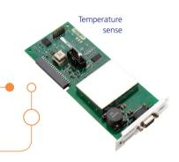
Expansion cards include additional temperature sensor inputs and heater outputs, pressure transducer inputs, stepper motor drive allowing gas flow regulation and efficient use of liquid helium in flow cryostats and cryogen level metering of both helium and nitrogen.
